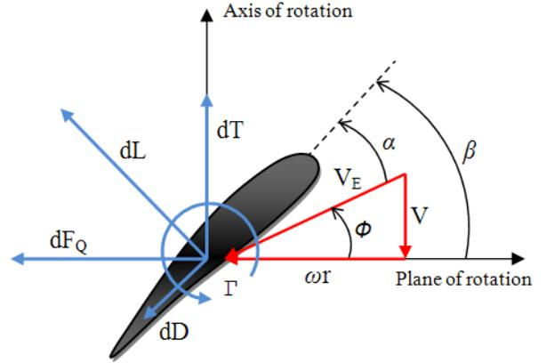
Figure 6: Vector diagram for a section  $dr$  a length  $r$  away from centre of the propeller
