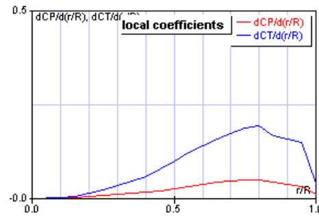
Figure 12: Change in  $C_P$  and  $C_T$  over the length of the propeller blade
