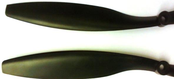
Figure 2: Counter-rotating fixed pitch propellers used for the quadrotor
