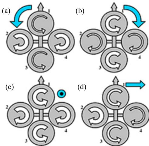
Figure 3: Quad-rotor dynamics, (a) and (b) difference in torque to manipulate the yaw angle ( $\psi$ ); (c) hovering motion and vertical propulsion due to balanced torques; and (d) difference in thrust to manipulate the pitch angle ( $\theta$ ) the roll angle ( $\phi$ ).
