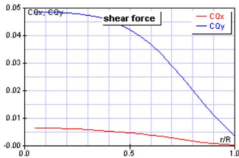
Figure 14: Graph of co-efficient of shear force VS relative radius
