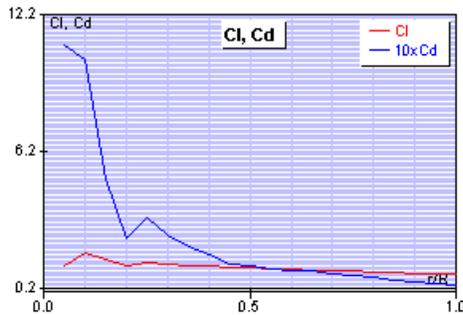
Figure 9: Graph of  $C_L$  and  $C_D$  VS relative radius
