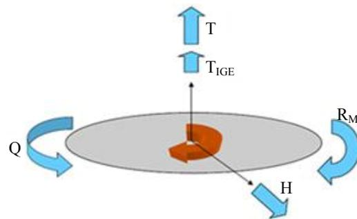
Figure 4: Aerodynamic forces and moments on a rotor
