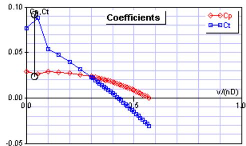
Figure 11: Graph of  $C_P$  and  $C_T$  VS advance ratio
