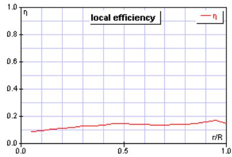
Figure 10: Graph of local efficiency VS relative radius
