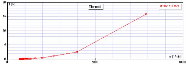
Figure 7: Graph of thrust VS rotor speed
