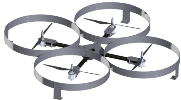
Figure 1: Proposed quadrotor structure
