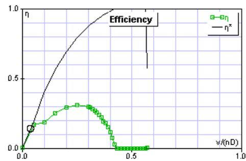
Figure 13: Graph of efficiency VS advance ratio
