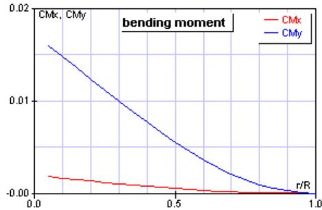
Figure 15: Graph of bending moment co-efficient vs relative radius
