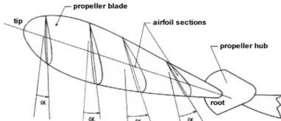
Figure 5: Typical fixed pitch propeller geometry
