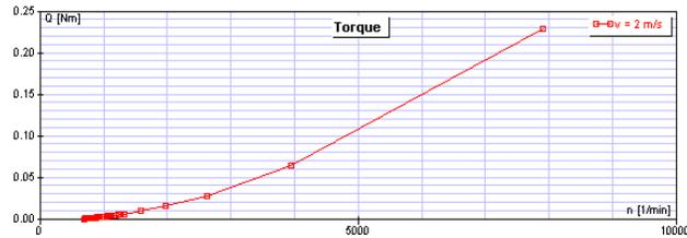
Figure 8: Graph of drag moment VS rotor speed
